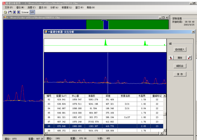
Fig. 5 Gamma-4 energy spectrum analysis software interactive analysis interface
